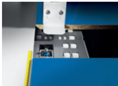
Infeed stop Pneumatically controlled. With EDGETEQ S-500.
