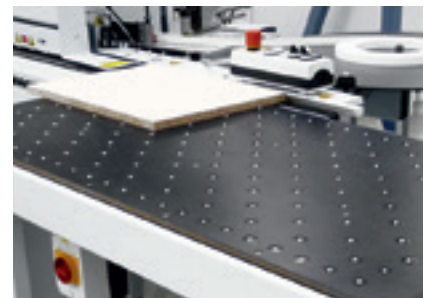
Air cushion table For easy workpiece feeding.
