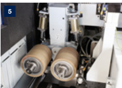
5 Top pressure rubber rollers for sensitive surfaces after processing (Shore hardness: 80)
