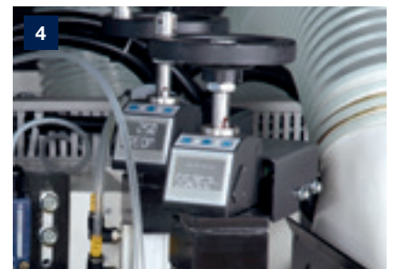
Review radial position of tools via electronic display including target value
