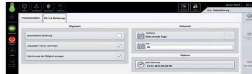
The integrated **backup system** logs all data of the machine periodically.
