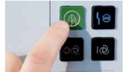
The **ecoPlus-Button** disrupts production and takes the machine into its energy-saving mode.
