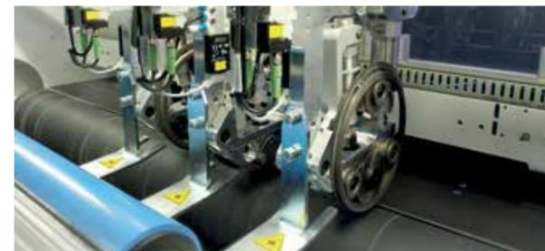
**Tools running on rubber rollers** provide for lower cutting force and lower wear-and-tear, at best cutting quality and long tool life.
