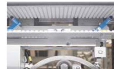
The **Tool-collision monitoring** prevents any collision and, therefore, tools or cardboard blanks from any damage.
