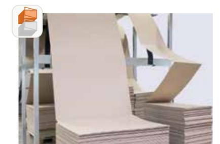
In the **Side by Side** operating mode, the cardboard feeding compartment is expanded by one more web width, allowing single sheet access to up to twelve web widths in a sixcompartment change system.
