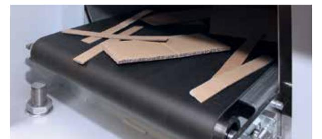
**Automatic removal of cutting scraps** enhances process reliability and reduces machine downtimes.
