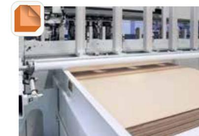
**The automatic single sheet feeder with lift table** allows the automatic feeding of stacked single sheets.
