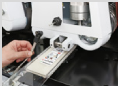
Quality in detail For example, the sanding elements with quick coupling for the grounding strap. Ensures operational safety and good sanding results
