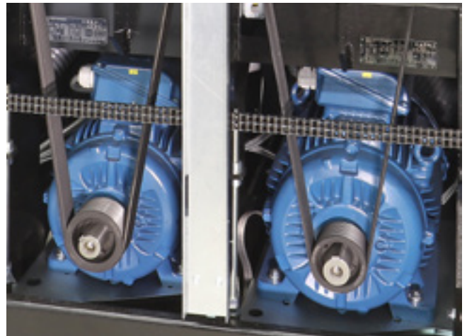
Separate drive motor for each head
