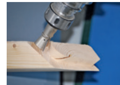
Dovetail at the jack rafter
