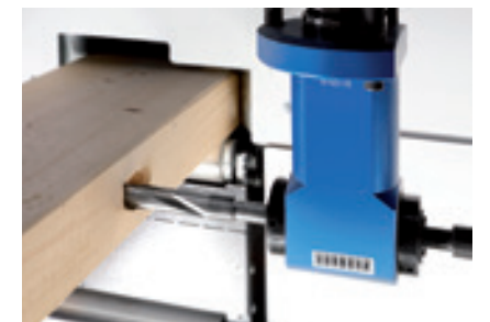
Production of mortises and pockets
