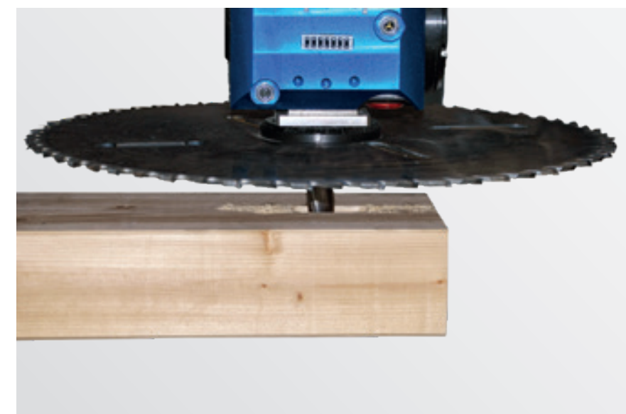
Saw blade with integrated routing unit
