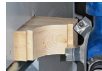
Machining the rafter head
