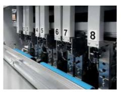
By means of **fully automatically movable and quickly repositioning cutting tools**, almost any blank can be produced.
