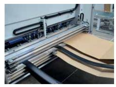
The PAQTEQ C-250, for example, can produce the **optimal cardboard box** – without much retooling – choosing fully automatically from up to twelve web widths.
