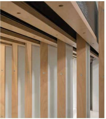
Pressing surfaces with tolerance compensation: The pressing lamellas work as a unit; they are placed on rubbers and suspended. Pressure is very evenly distributed due to the fact that the pressing lamellas simultaneously impinge on the carcass. Tolerances in the carcass are better absorbed.
