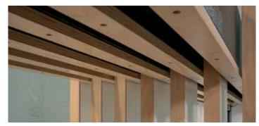
**Pressing surfaces with tolerance compensation**: The pressing lamellas work as a unit; they are placed on rubbers and suspended. Pressure is very evenly distributed due to the fact that the pressing lamellas simultaneously impinge on the carcass.
