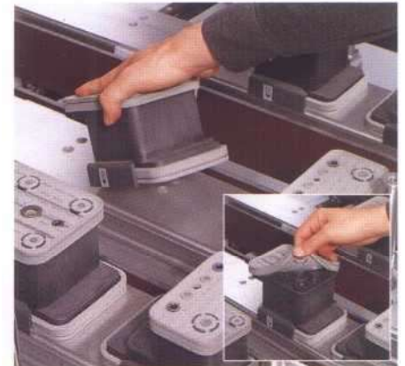
Easy exchange of the rubber pod cover
