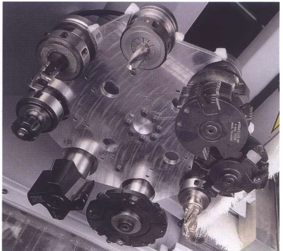
8-fold magazine in X- and Y-direction ride along
