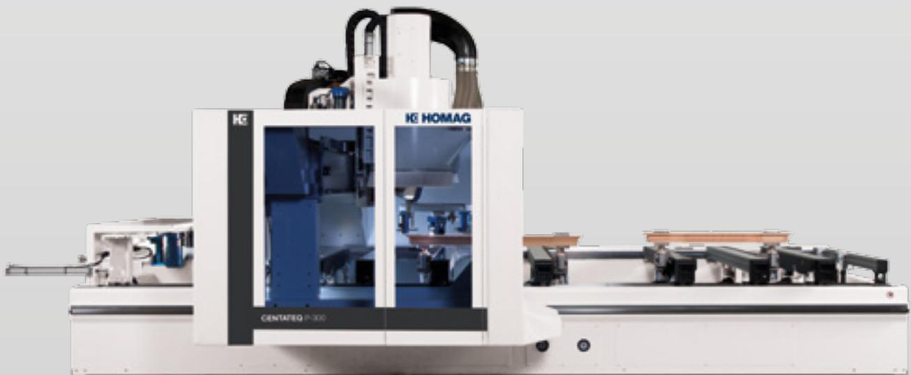
**CENTATEQ P-300:** Processing centre with 3-step clamping system for window manufacturing
