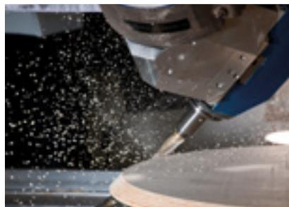
Chamfer trimming on a table top
