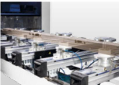
**powerClamp:** Manual clamping fixture powerClamp for straight and curved parts. Ideal for all arched, narrow and frame parts.
