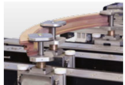
**3-step clamp:** Highly rigid 3-step clamps with extreme clamping height for precise complete processing of window and front door components without subsequent outside moulding and profiling.
