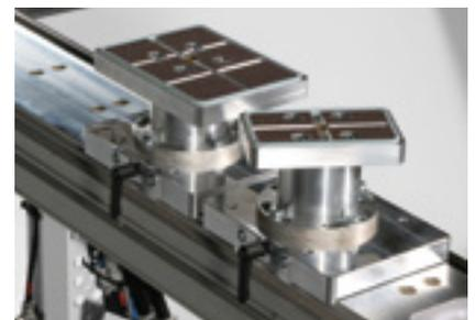
**Vacuum clamps made of aluminum:** Vacuum clamp in aluminium with additional mechanical clamping operation at the console for engaging solid wood parts. The suction plate can be rotated and also exchanged, and is lined with emery cloth.
