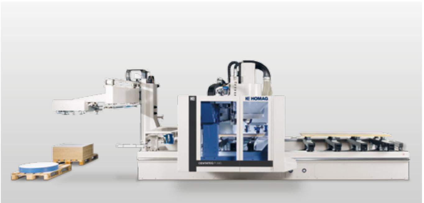
**TBA feeder attachment:** Simple, space-saving entry into the world of automation with the TBA feeder attachment mounted laterally at the machine. Reliable handling, precise positioning and integrated workpiece cleaning. Extreme operating and programming simplicity through direct use of the woodWOP processing program.
