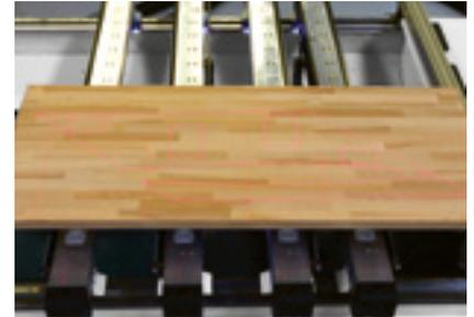
**Laser projection** of the clamps and the workpiece contour for optimum utilization and simple positioning of raw parts which cannot be aligned at the stops.
