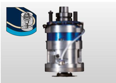
**Vertically traced trimming unit:** By means of a tracing ring with dia. 70 mm / dia. 130 mm, or tracing pad, it is possible to perform operations such as pocket trimming in precise relation to the workpiece surface. When connecting kitchen worktops, tracing guarantees an offset-free transition by precise trimming of grooves for the tongue and groove joint.
