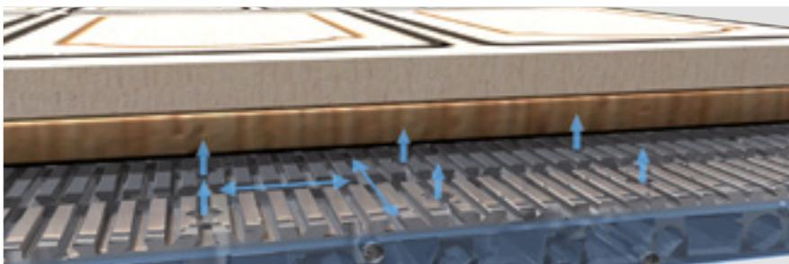
**Vacuum grid table with air cushion function:** The vacuum transmission is integrated in the design of the aluminium grid table. Division into zones and efficient vacuum pumps ensure reliable clamping, even for nesting processes with underlay panels. The air cushion function makes light work of handling large-format panel-shaped workpieces.
