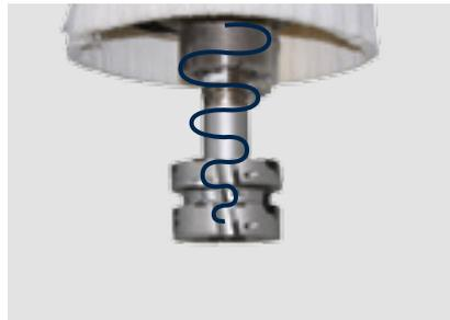
**Fluid cooling and spindle sensor:** Fluid-cooled trimming spindles with hybrid bearings offer a long service life. An additional vibration sensor detects tool imbalance and protects the spindle from overload, for instance due to excessively high feed rates.
