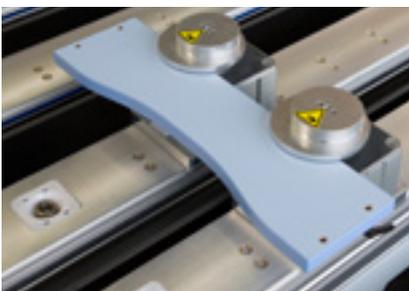
**Multiclamp for dual circuit vacuum system:** Vacuum actuated clamping element for clamping strips and staves
