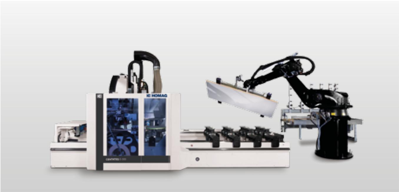
**Robot handling systems:** Unlimited workpiece handling with different layer patterns, storage positions, alignment and flipping. Supplementary functions such as labeling, position measurement or cleaning can be simply integrated.
