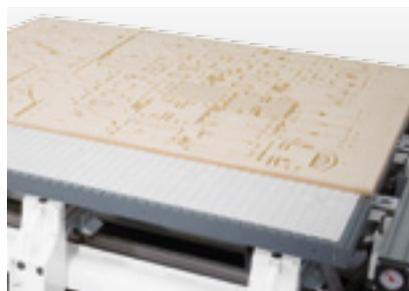
**Matrix adapter plate:** Highly flexible clamping systems offer secure fixture even when working with filigree workpieces. The matrix adapter panel even permits shaped components to be “cut to size” with optimized cutting waste on a console table machine using the nesting process.
