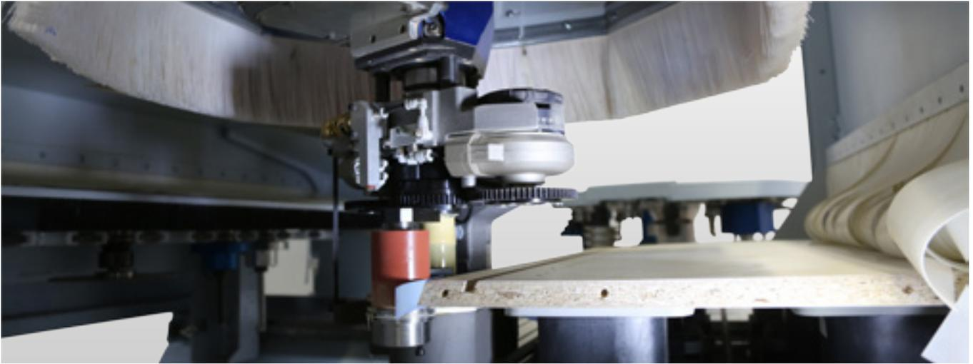
**easyEdge and DRIVE5C+:** The perfect combination of edge gluing and high-performance 5-axis processing. The DRIVE5C+ spindle engages the easyEdge unit directly from the pickup station in the lateral linear changer, the edging material is fed in – done.
