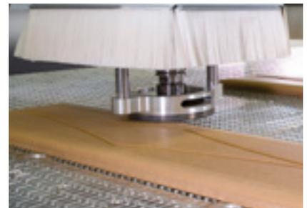
**sensoflex tracing system:** Perfect workpiece quality – the traced spindle compensates for unevenness and unwanted tolerances. Tracing facility for different tools ensures complete flexibility
