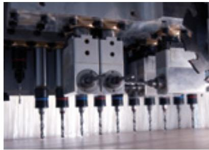
High-speed drilling technology with grooving saw
