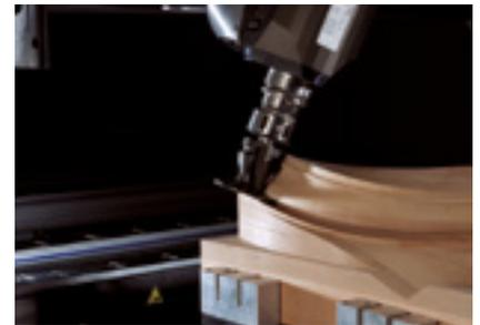
Routing of a stair hand rail
