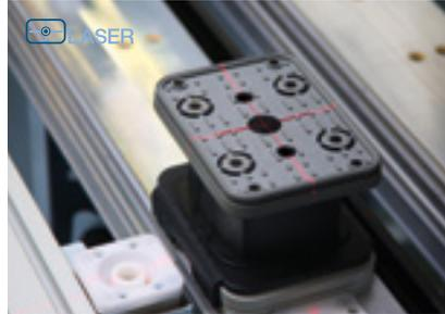
**Suction cups** are displayed using a laser beam (cross hairs). The workpiece contour can be “travelled” as a positioning aid for freeform part.
