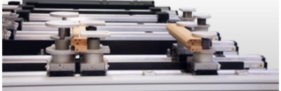
**powerClamp:** powerClamp clamping fixture for straight and curved parts. Ideal for all arched, narrow and frame parts. Also with automatic reclamping for 5-sided processing.
