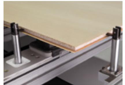
**Bolts with end position scanning and for laminate overhang:** Stop bolts with end position monitoring to protect tools, units and machine operating staff. Exchangeable stops specifically for workpieces with laminate overhang.
