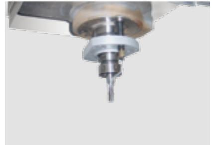
**Minimum quantity lubrication:** Machining of aluminium with minimum quantity lubrication through the unit or by means of an external spray pipe at the spindle for maximum care of tools.
