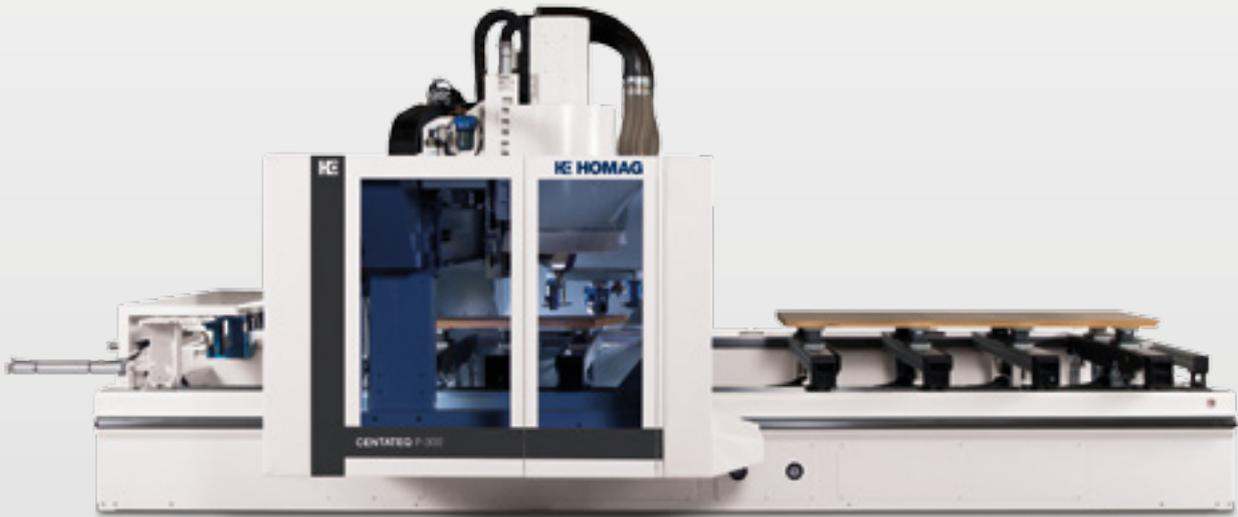
**CENTATEQ P-300:** Processing center with five axis spindle for universal processing in joinery and general woodworking
