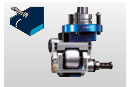
**Horizontally traced trimming unit:** By means of a tracing roller, horizontal trimming operations are performed precisely relative to the workpiece surface, e.g. during flush trimming of overhanging edges on the postforming profiles of a kitchen worktop. The diameter of the tracing roller and trimming tool are coordinated, generally to 20 mm.
