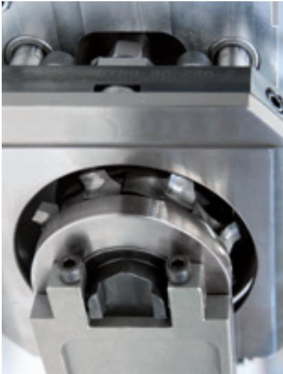
**flexTrim am Formfräsaggregat**
