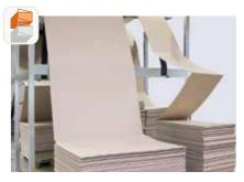
In the Side by Side operating mode, the cardboard feeding compartment is expanded by one more web width, allowing single sheet access to up to twelve web widths in a sixcompartment change system.
