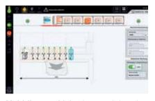
Multi-line machining by way of six real and six additional virtual longitudinal tools as well as a transverse tool allow for more complex cutting of blanks and packaging design.
