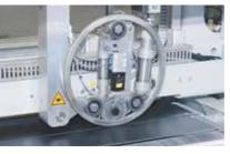
Service features: After each change of tools, the new tools are automatically calibrated. After cutting 100 blanks, tools are dynamically and automatically repositioned inorder to minimize the wearand-tear of the rubber roller.
