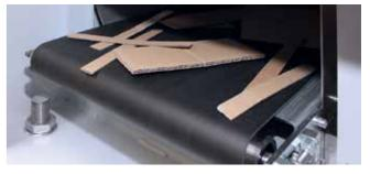
Automatic removal of cutting scraps enhances process reliability and reduces machine downtimes.
