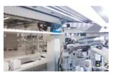
Permanent positioning monitoring of the longitudinal tools and automatic positioning correction safeguard the design-relevant process and the execution of cuts.
