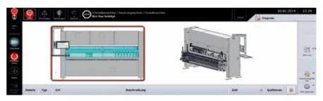
The integrated troubleshooting system analyses all work processes, reports necessary maintenance, the replacement of wear-and-tear parts (cutting blades), and the like, in order to guarantee consistently high quality and to avoid downtimes.
