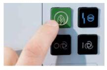
The ecoPlus-Button disrupts production and takes the machine into its energysaving mode.
