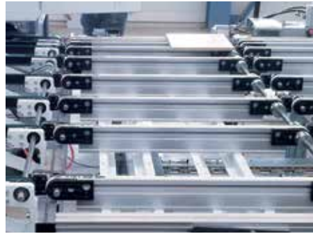
Small roller gib to support long transverse workpieces (option)
