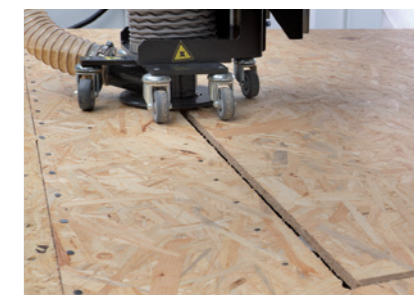
WALLTEQ M-320: fully automatic processing with the routing unit
