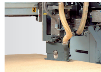
WALLTEQ M-300: fully automatic processing with the sawing unit
