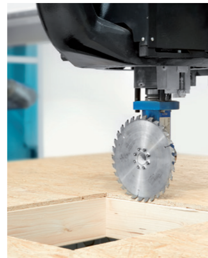
Manufacturing window openings
