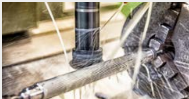
Milling of drive roll
