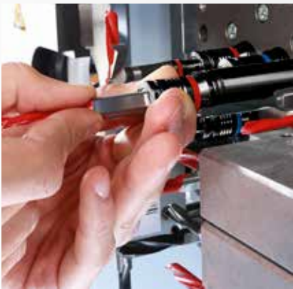
Configuration choice B: Drill quick-change system Quick-change system for a drill change without tools to reduce setup times.
